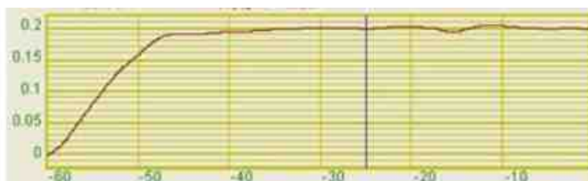
Regulator program - optimal integral factor
