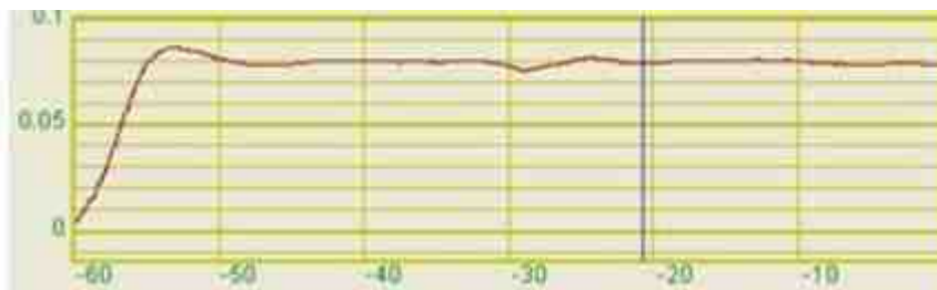
Regulator program - process with optimal differential ratio
