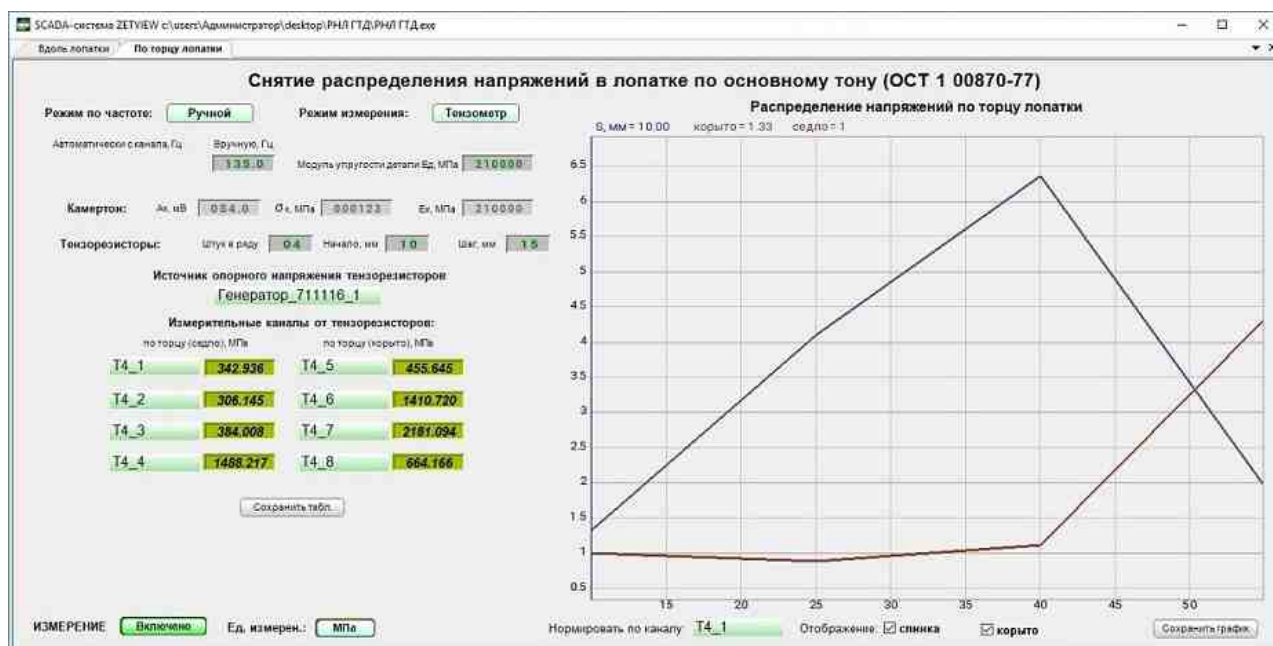
Fig. 17.11 Tab "At the end of the blade" of the program window "SDS_GTE(ZET058)" during measurements
