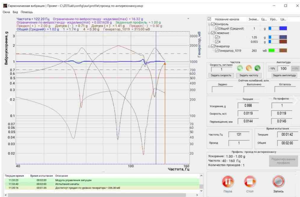
Fig. 7. Passage of vibration testing through two control channels
