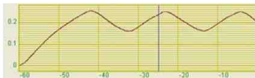
Regulator program - the integral ratio is too high - the signal reaches the self-oscillations mode
