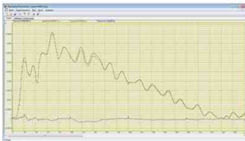
Fig. 3 — shock spectra: instantaneous, averaged and their difference
