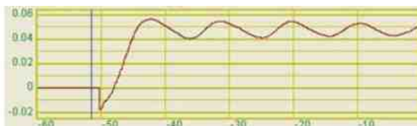
Regulator program - presence of undamped oscillations in the signal
