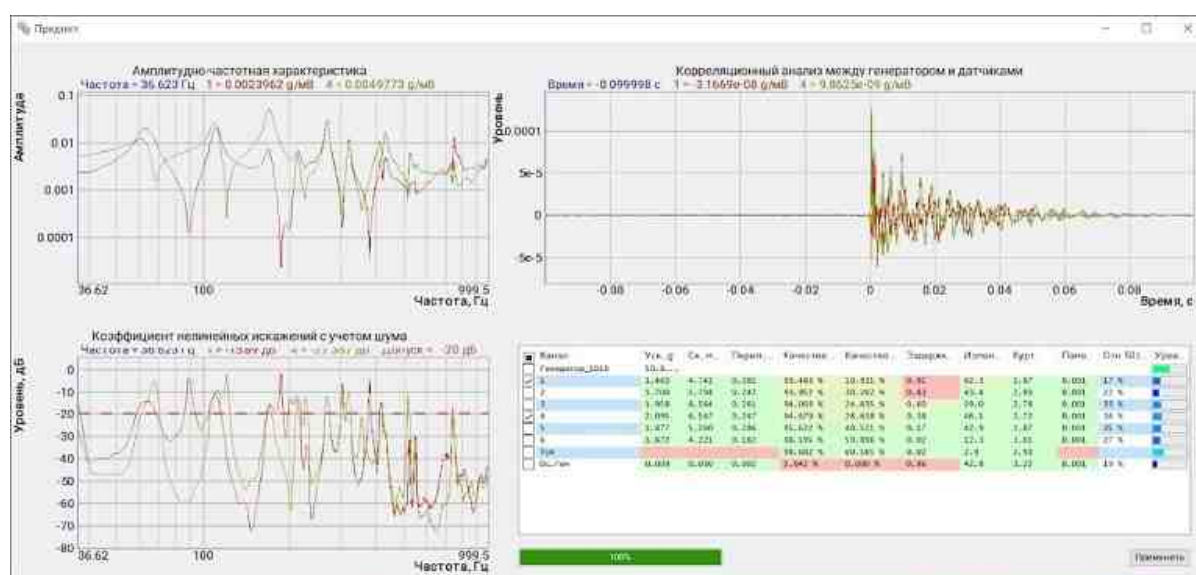
Fig. 8.16 Results of the Pre-Test for two sensors installed in the wrong places
