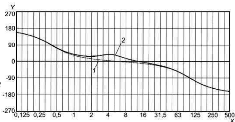
X - frequency, Hz; Y - phase, °; 1 - bandpass filter; 2 - frequency correction function W_j
