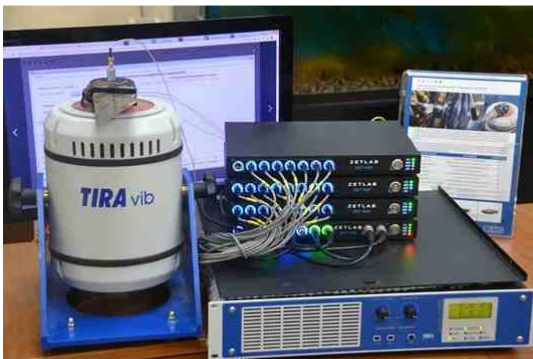
Fig. 17.8 Equipment set for removal of stress distribution in the blade
