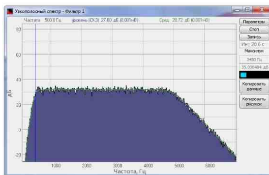
Bandpass filter F_{\text{cutoff HPF}} = 500 \text{ Hz} ; F_{\text{cutoff LPF}} = 5000 \text{ Hz}
