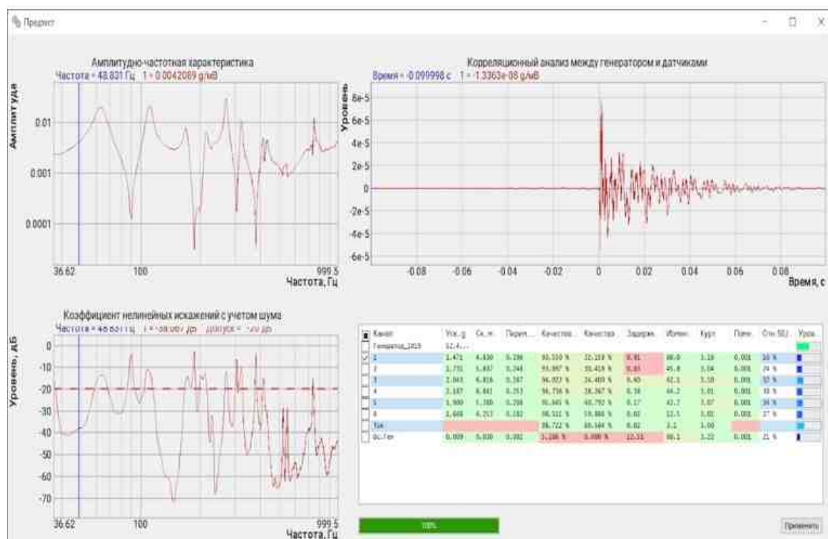
Fig. 8.13 Results of the Pre-Test for a sensor mounted on the edge of the test object
