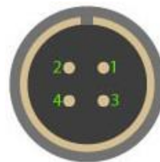
FQ14-4TJ-7 connection of the cable
