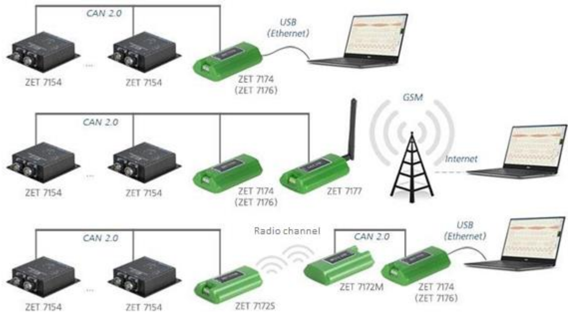
Figure 2.7 Variants of establishing measuring lines with CAN interface
