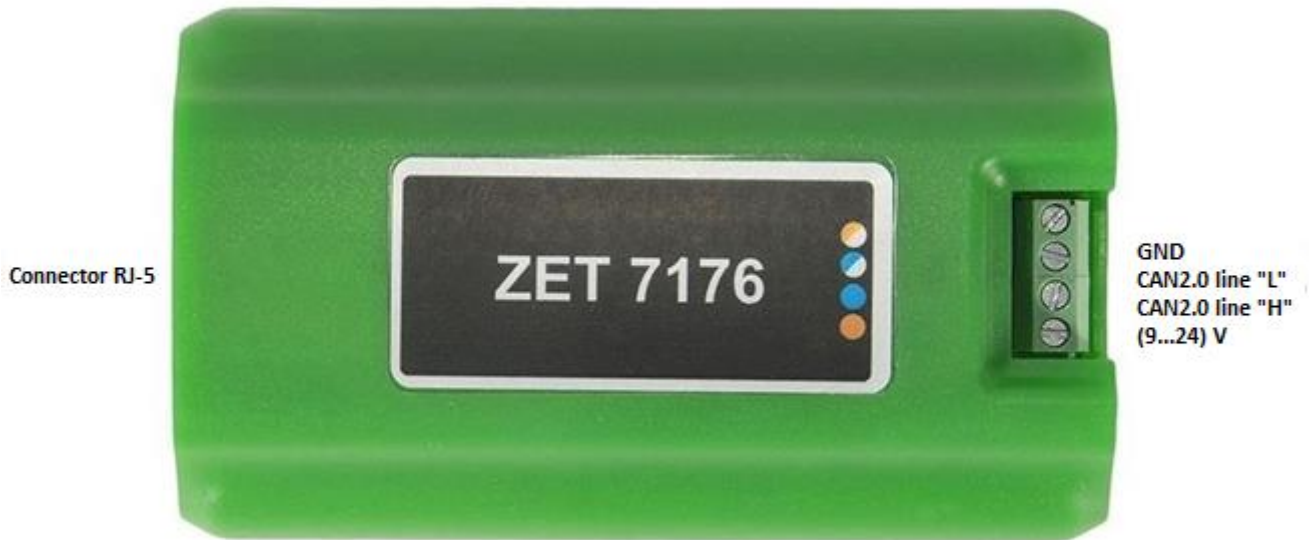
Figure 2.3 Contacts labelling of ZET 7176 (laboratory version)
