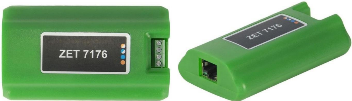
Figure 2.1 External view of the interface converter (laboratory version)
