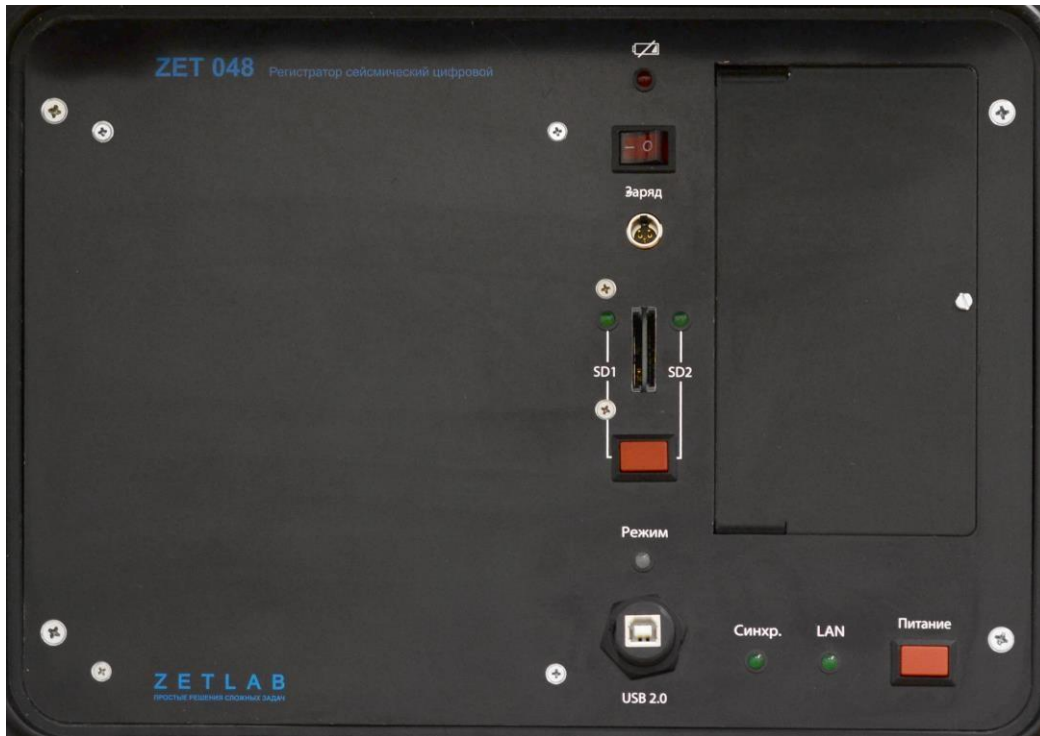
Figure 1.3 ZET 048-E recorder control panel
